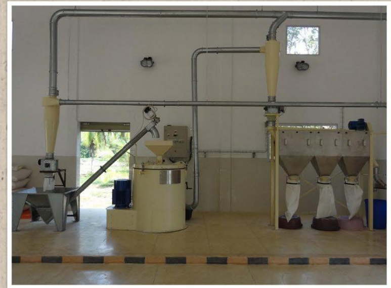
Simple Rice Plant for Polished Rice 250 kg/hr Fine, White Rice Meal 180 my
