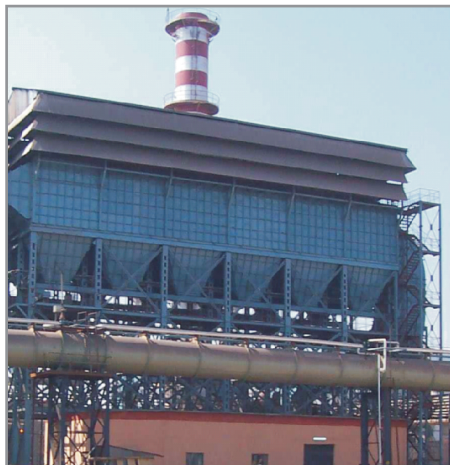
Specialised Dedusting system in a cast house
